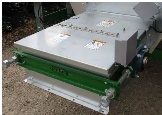
Image 30 – Conveyor tail section door
