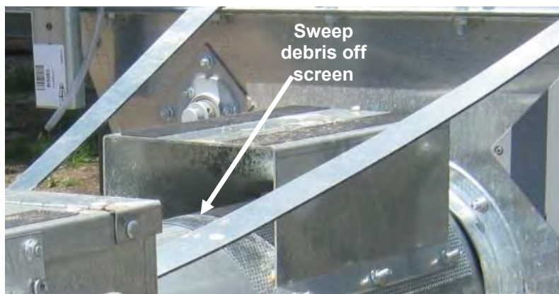
Image 4-41 – Grain discharge chute screen
