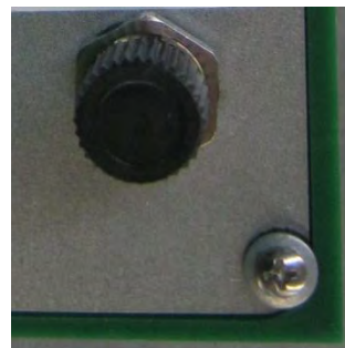
Image 4-52 – Cable connector capped
