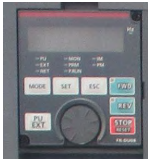
Mitsubishi F800 control panel
