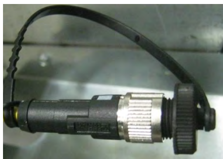
Image 4-51 – Moisture sensor cable capped
