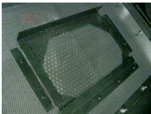
Image 23 – Inner grain column cleanout door
