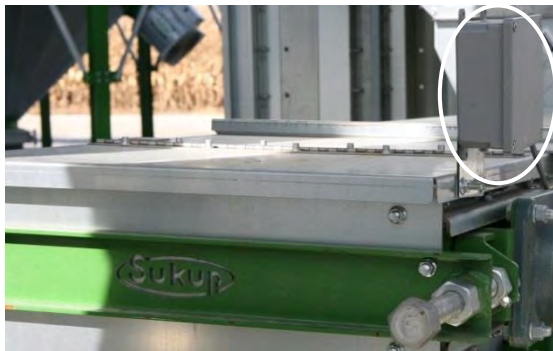
Image 4-28 – Grain discharge chute switch on drag conveyor unload system
