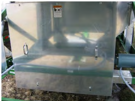
Image 29 – Unload auger/meter roll drive service door
