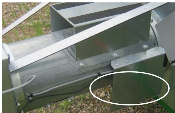
Image 4-2 – Discharge moisture sensor location on auger-unload dryer
