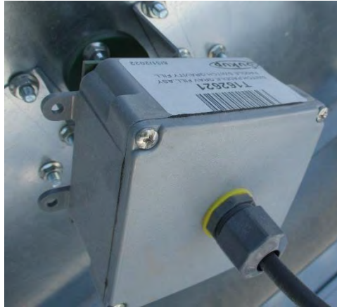
Image 4-8 – Paddle switch T162621 on gravity-fill section
