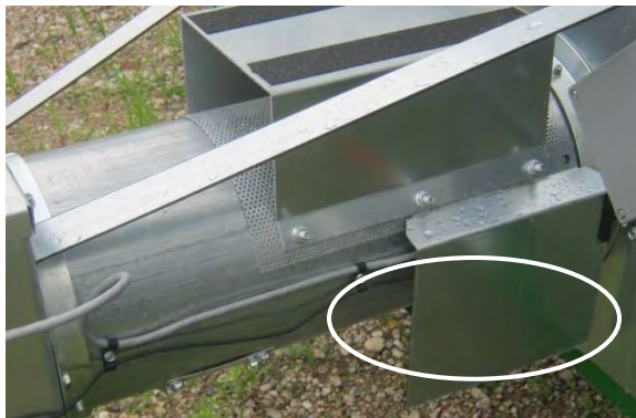
Image 19 – Discharge moisture sensor location
