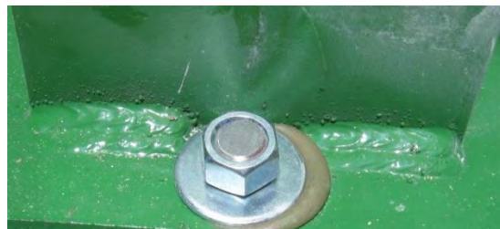
Image 2-2 – Anchor bolt on base weldment
