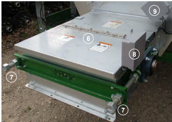
Image 7 – Components of conveyor tail
