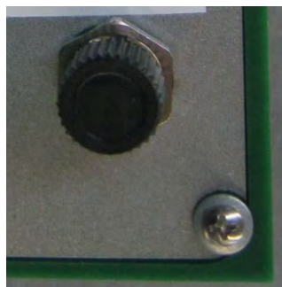
Image 4-3 – Cable connector capped
