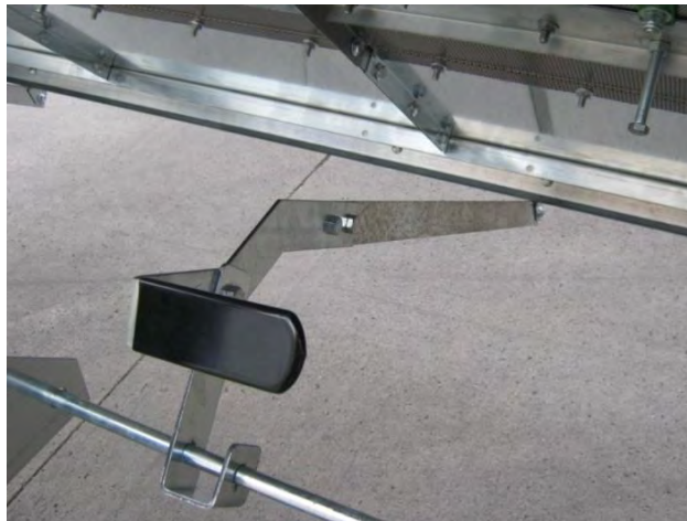
Image 4-46 – Unload auger outside access/cleanout door handle
