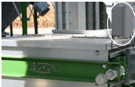
Image 5-2 – Grain discharge chute switch box on drag conveyor unload
