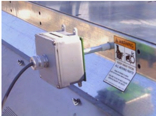
Image 4-30 – Paddle switch T16244 on auger-load section
