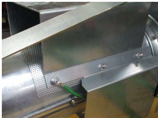
Image 2-22 – Grounding at discharge tube
