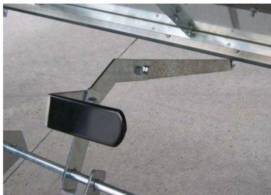
Image 24 – Unload auger cleanout door handle
