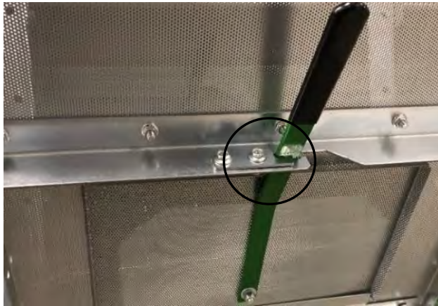
Image 4-48 – Outer grain column cleanout door
