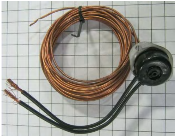
Image 5-14 – Grain column over-temp switch
