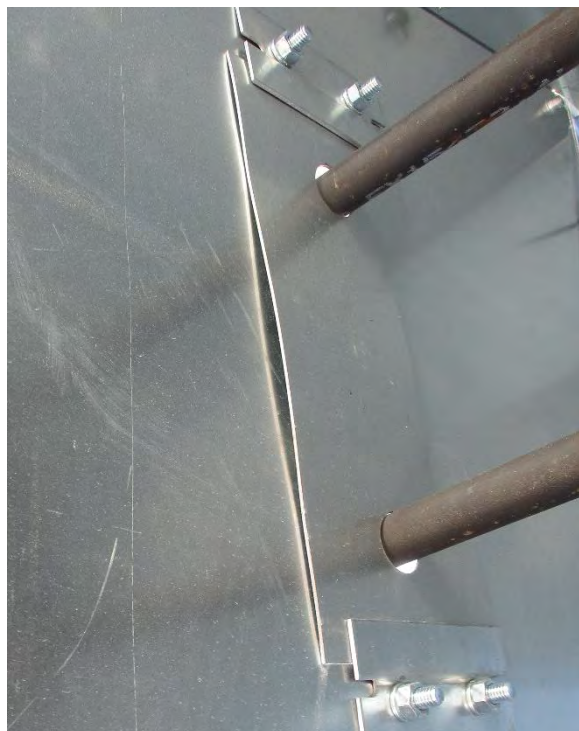
Image 3-2 – Vaporizer adjustment plate
