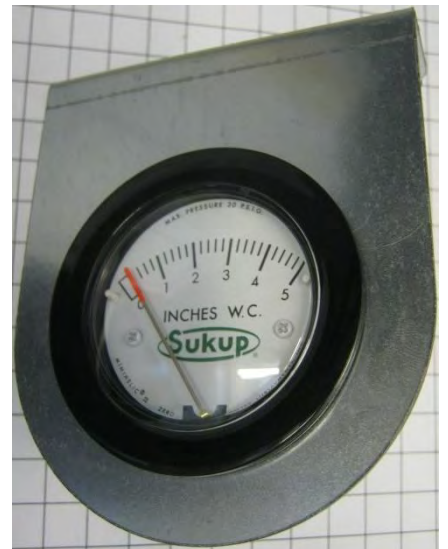
Image 3-7 – Vacuum pressure gauge
