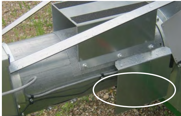
Image 4-1 – Discharge moisture sensor location on auger-unload dryer
