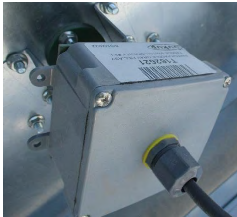
Image 4-9 – Paddle switch T162621 on gravity-fill section
