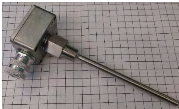
Image 5-25 – Single-point grain sensor RTD
