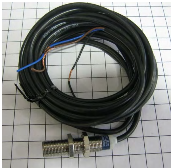
Image 5-16 – Sample box proximity switch
