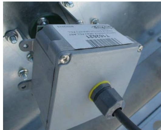
Image 5-6 – Paddle switch T162621 on gravity-fill section
