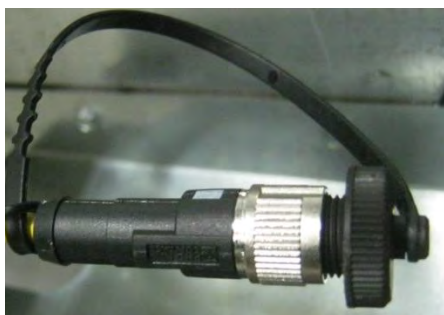
Image 4-48 – Moisture sensor cable capped
