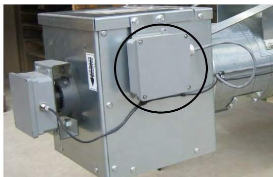
Image 5-2 – Grain discharge chute switch box on auger unload
