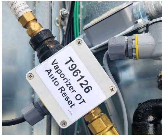
Image 4-11 – Vapor over-temp switch (shown on axial-fan dryer)
