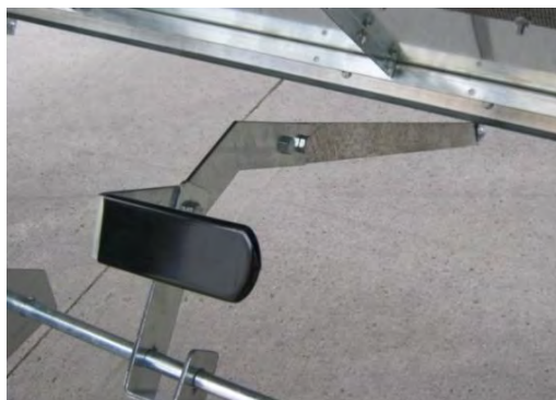
Image 26 – Unload auger cleanout door handle
