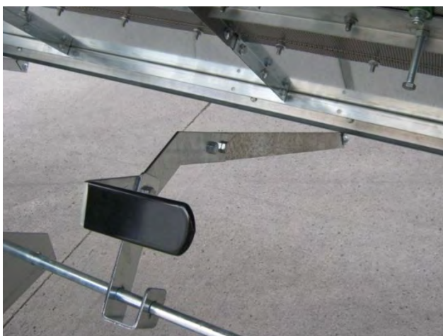
Image 4-42 – Unload auger outside access/cleanout door handle
