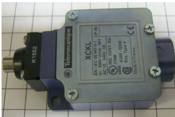
Image 5-12 – Rear door switch
