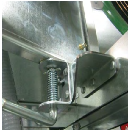
Image 3-5 – Spring pin on intake door
