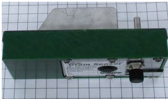
Image 5-22 – Discharge moisture sensor
