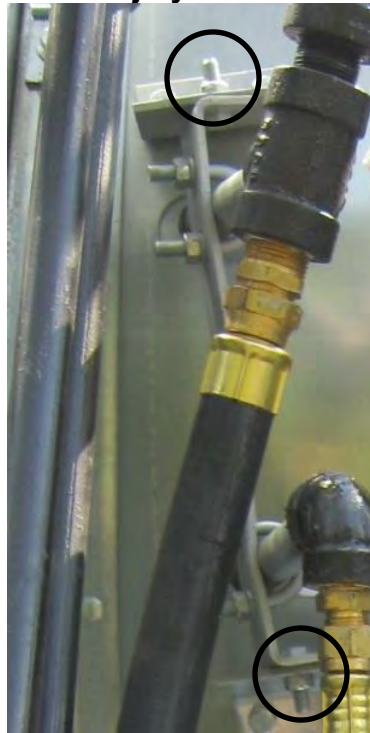
Image 3-1 – Vaporizer bracket on axial-fan dryer
