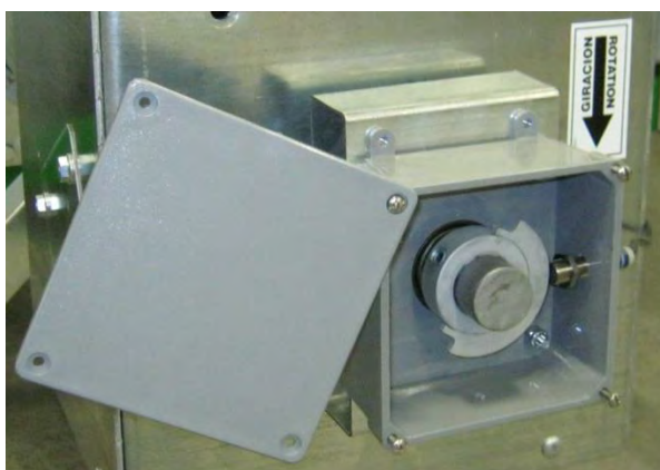
Image 19 – Unload auger proximity switch
