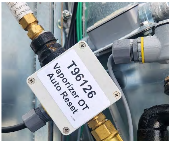
Image 5-9 – Vapor over-temp switch (shown on axial-fan dryer)
