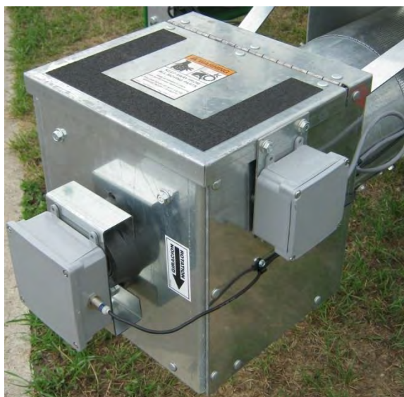
Image 32 – Unload auger service door
