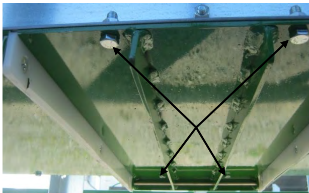
Image 4-43 – Drag conveyor cleanout door Remove bolts to open
