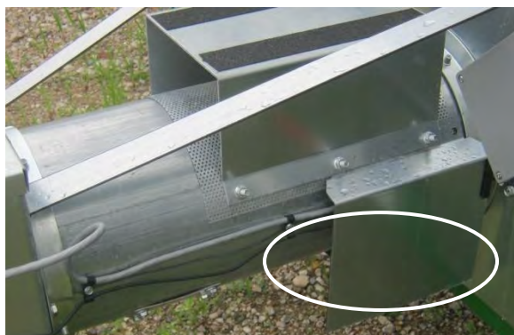
Image 4-38 – Discharge moisture sensor location
