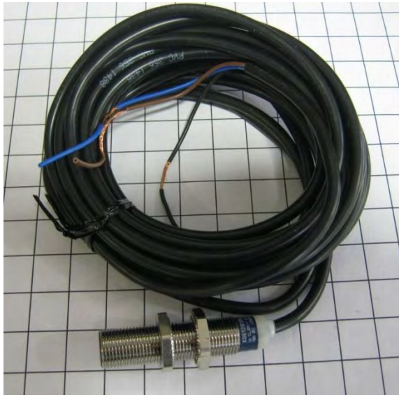
Image 5-7 – Unload auger proximity switch
