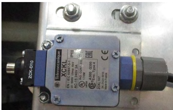
Image 18 – Rear door switch
