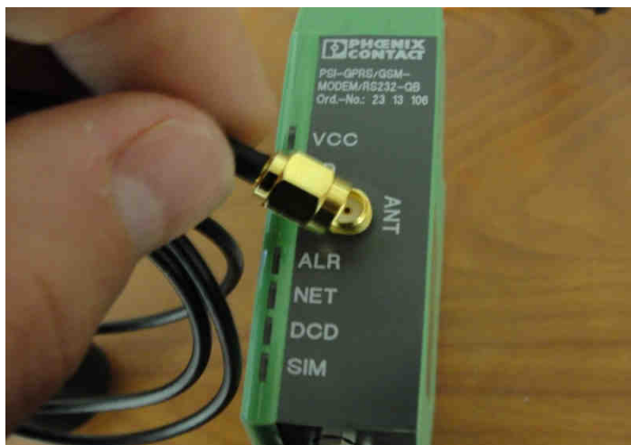
Image 6 – Plugging in antenna
