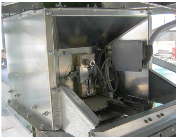
Image 4-10 – Discharge moisture sensor in static sample box
