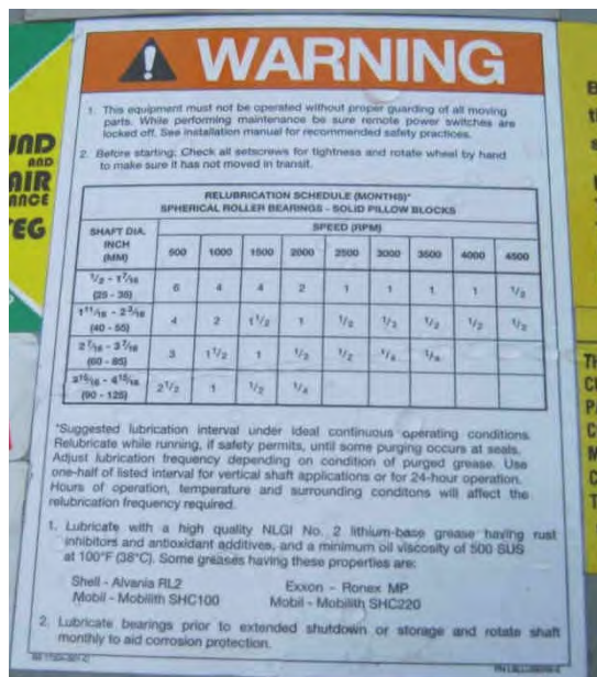
Image 3-2 – Twin City Fan & Blower lubrication sticker
