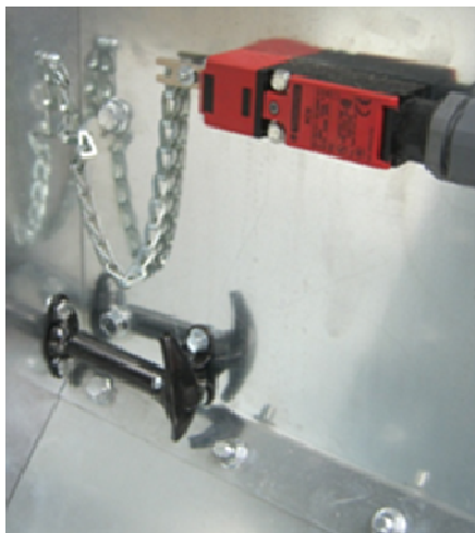
Image 4-5 – Access door switch
