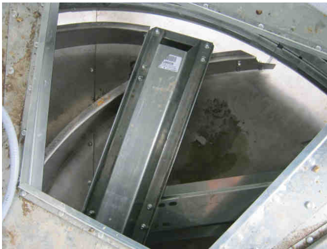
Image 18 shows rotor arm and scraper (curved) of unload.
