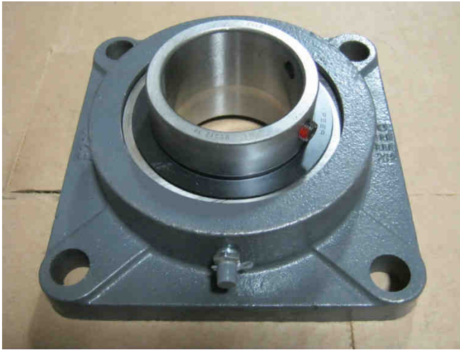
Image 3-11 – Bearing used on unload rotor
