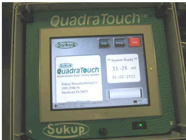
Image 33 – Main power switch on
