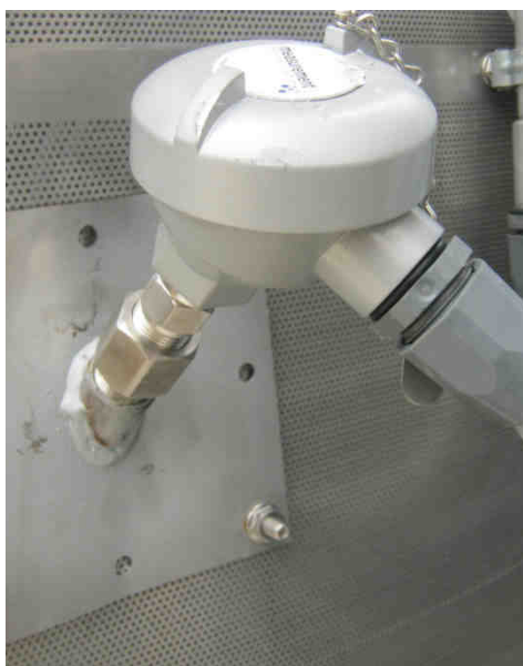
Image 4-12 – Single-point grain column temperature sensor
