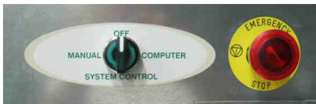
Image 11 – System Control switch and Emergency Stop switch
