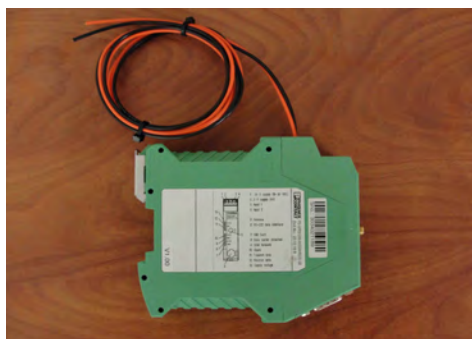
Image 3 – GSM modem power wires
