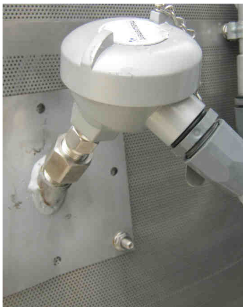
Image 14 – Single-point grain temperature sensor RTD
