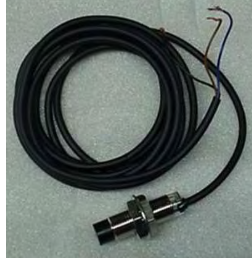
Figure 1.8b: Metering Roll Proximity Switch
