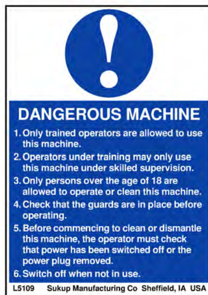
Label #L5109 – Place near main power panel.
