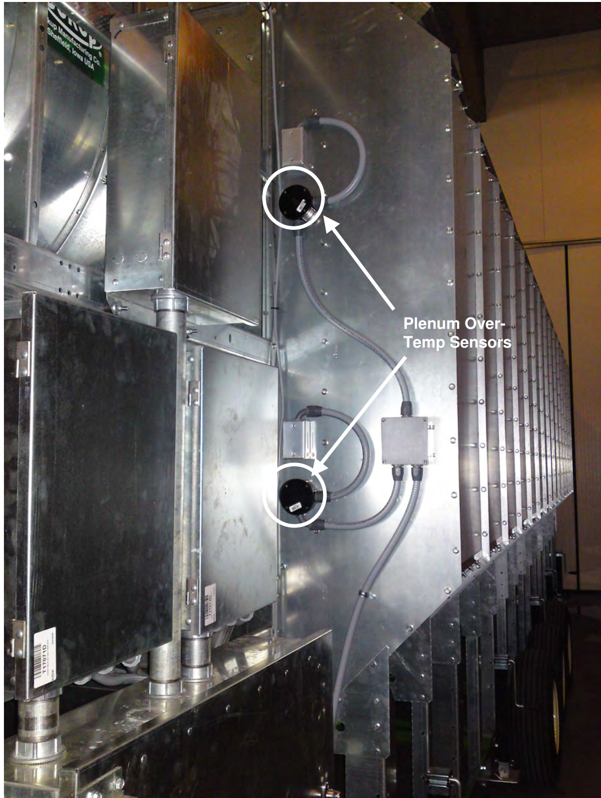
Figure 1.10c: Plenum Over-Temperature Sensors Installed on Dryer (Located in same box as Static Air Pressure Sensor.)
