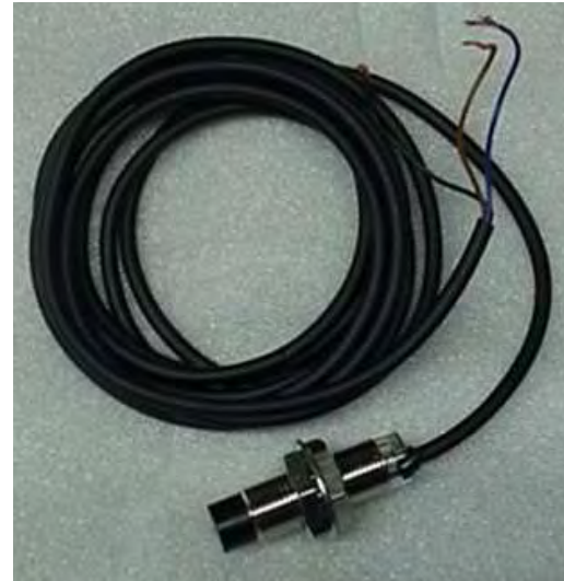
Figure 1.8b: Metering Roll Proximity Switch
