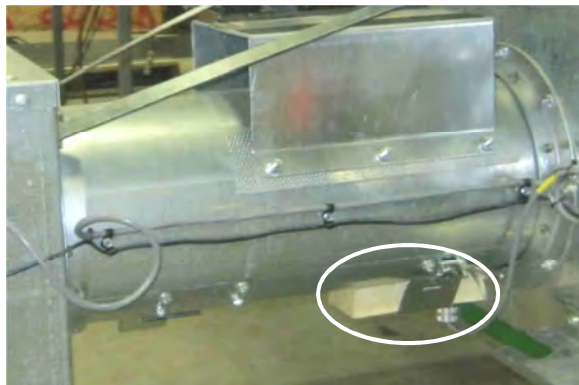
Image 4-28 – Discharge moisture sensor installed
