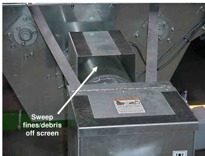
Image 4-27 – Grain discharge chute screen
