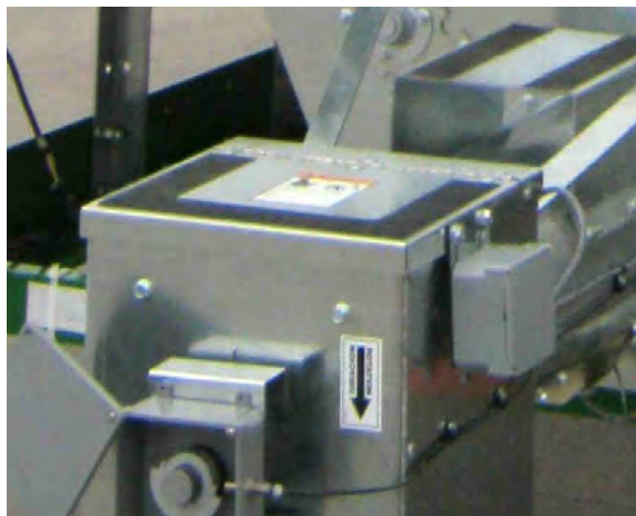
Image 41 – Unload auger service door
