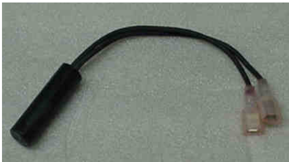
Image 5-1 – Grain discharge chute switch
