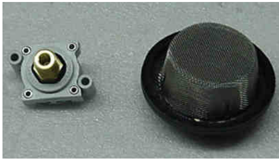
Image 5-17 – Static air pressure switch disassembled. See Image 5-18 (Item 2) for location of air switch.
