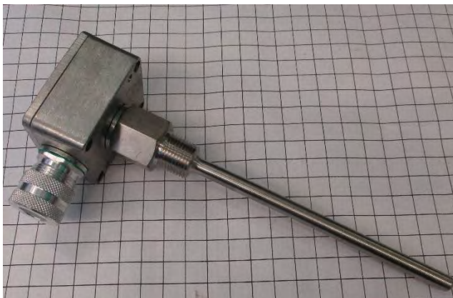
Image 4-12 – Single-point grain column temperature sensor
