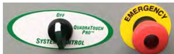
Image 3 – System Control & Emergency Stop switches
