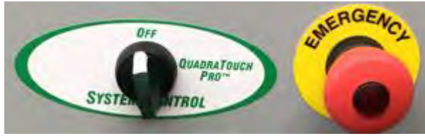
Image 2-1 – System Control switch, Emergency Stop button
