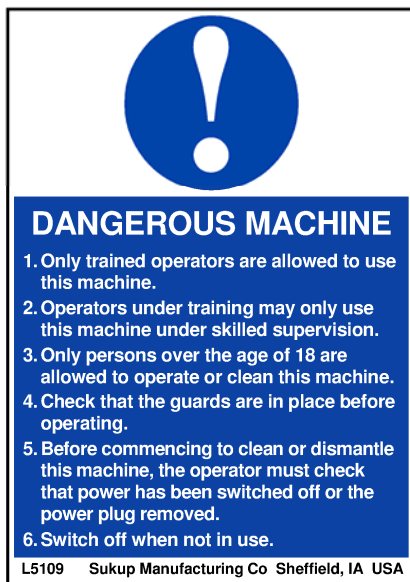
Label #L5109 – Place near main power panel.
