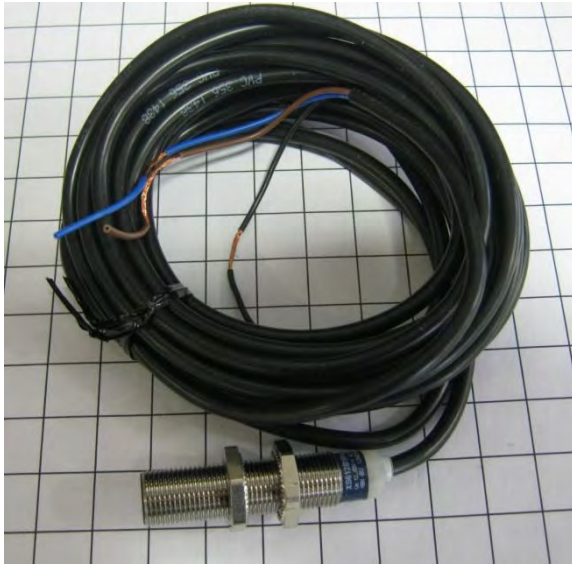
Image 5-19 – Sample box proximity switch
