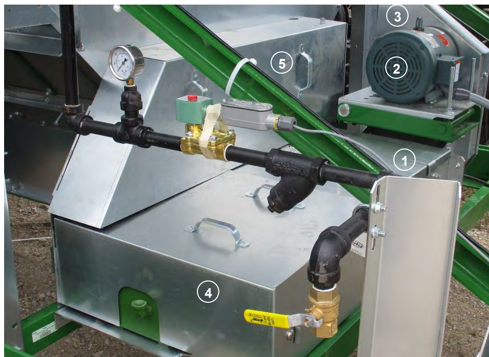
Image 6 – Components of head of unload conveyor
