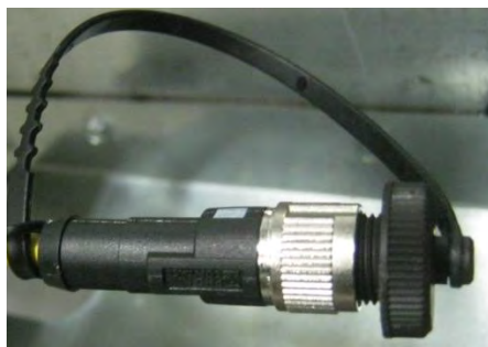
Image 4-52 – Moisture sensor cable capped
