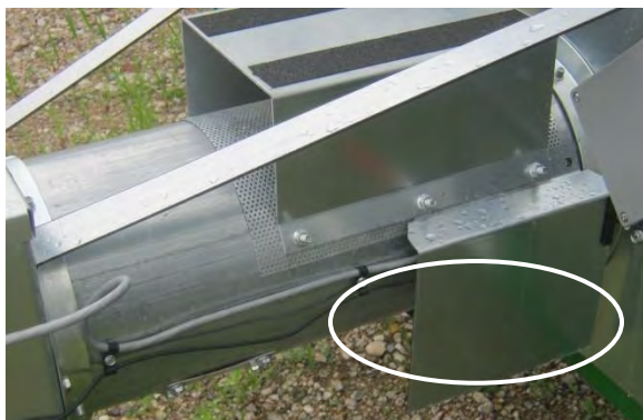
Image 19 – Discharge moisture sensor location
