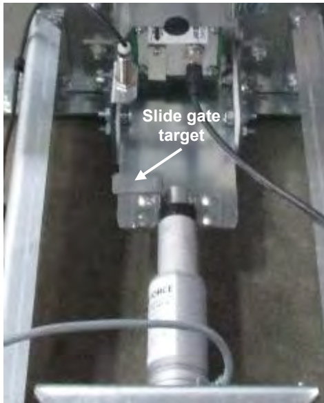
Image 4-12 – Actuator for static sample box slide gate
