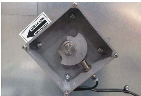
Image 28 – Meter roll proximity switch
