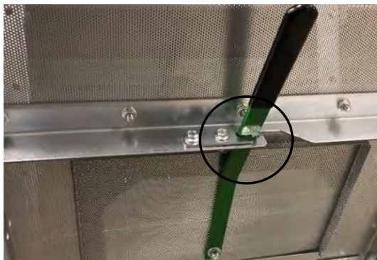
Image 22 – Outer grain column cleanout door
