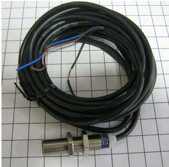
Image 5-21 – Unload auger proximity switch
