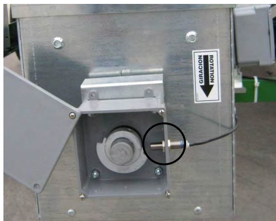
Image 4-25 – Unload auger proximity switch
