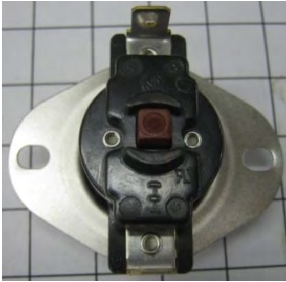
Image 5-16 – Heater housing high-limit switch
