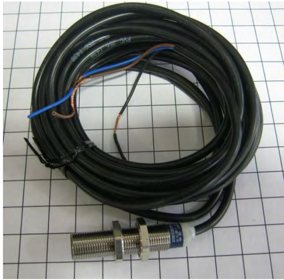
Image 5-17 – Meter roll proximity switch
