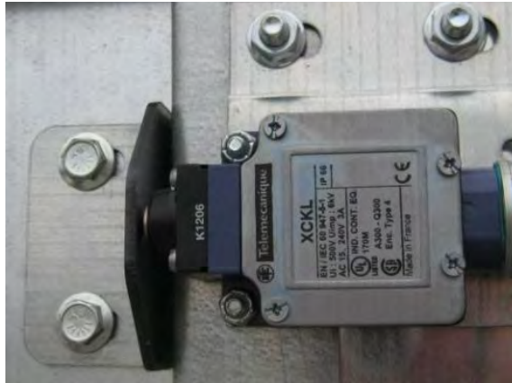
Image 4-14 – Rear door switch
