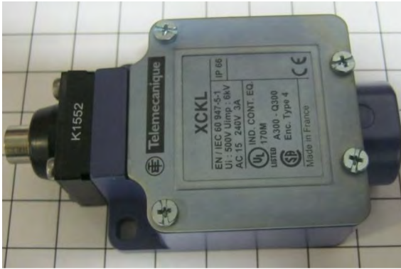
Image 5-12 – Rear door switch
