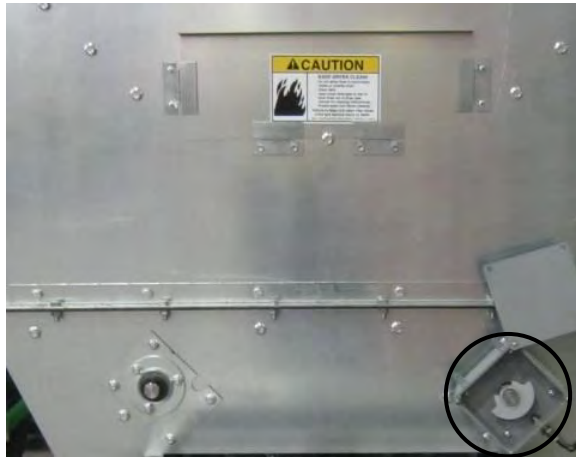
Image 4-19 – Meter roll proximity switch
