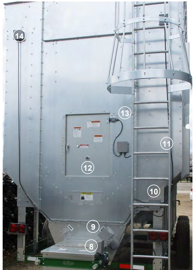
Image 5 – Back of dryer w/ conveyor unload
