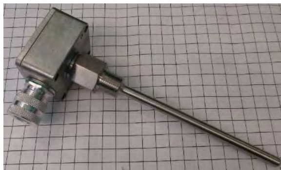
Image 5-29 – Single-point grain column RTD sensor
