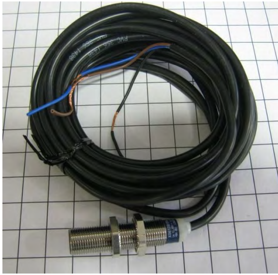
Image 5-7 – Unload auger proximity switch
