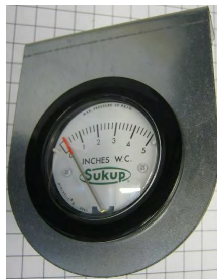
Image 3-7 – Vacuum pressure gauge
