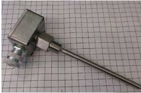
Image 4-22 – Single-point grain temp sensor
