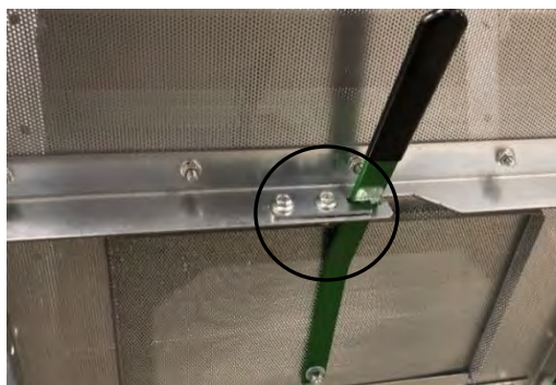
Image 23 – Outer grain column cleanout door
