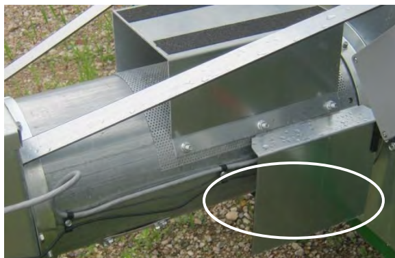
Image 5-23 – Discharge moisture sensor location
