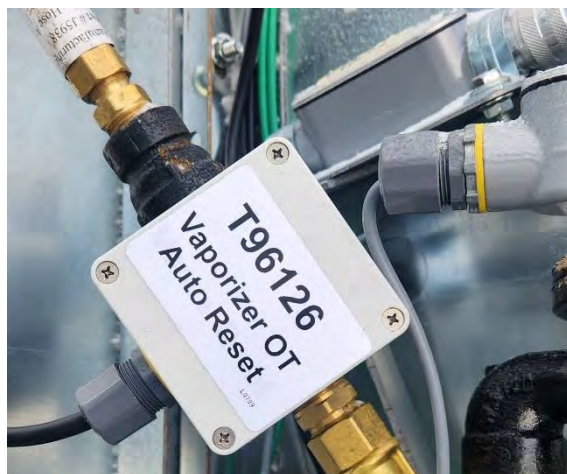
Image 5-9 – Vapor over-temp switch (shown on axial-fan dryer)
