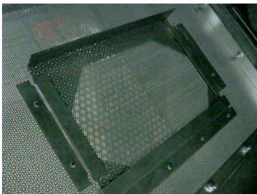
Image 24 – Inner grain column cleanout door
