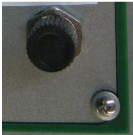
Image 4-3 – Cable connector capped
