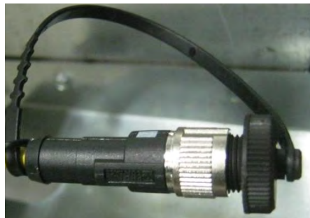
Image 4-48 – Moisture sensor cable capped
