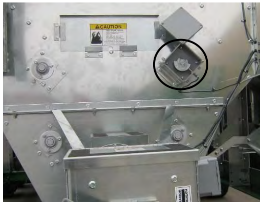
Image 5-15 – Meter roll proximity switch
