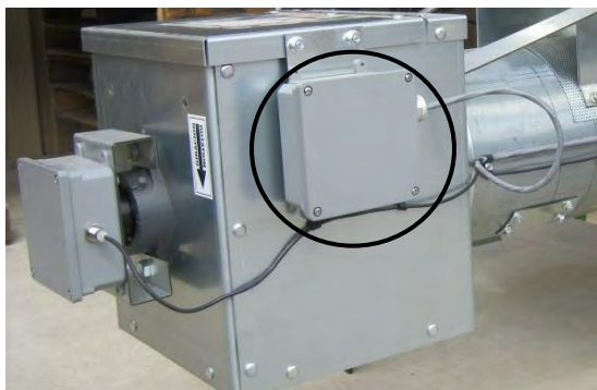
Image 5-2 – Grain discharge chute switch on auger unload
