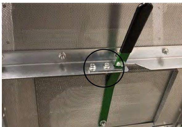
Image 4-45 – Outer grain column cleanout door
