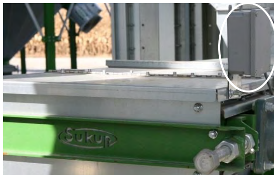
Image 4-6 – Grain discharge chute switch on drag conveyor unload system
