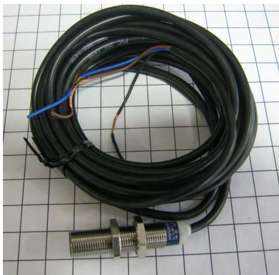
Image 5-16 – Sample box proximity switch
