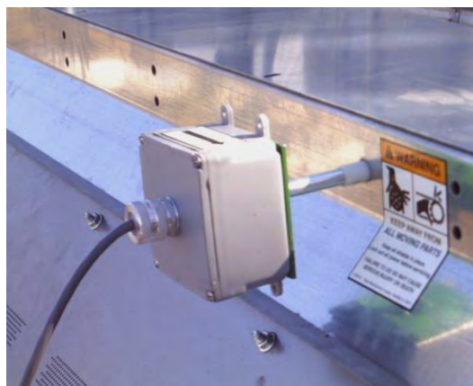
Image 5-5 – Paddle switch on auger-fill section
