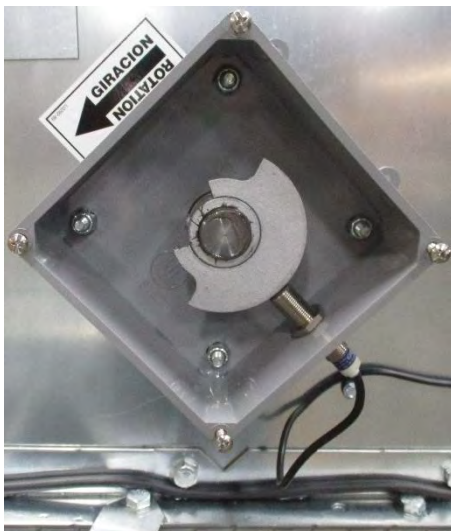
Image 29 – Meter roll proximity switch
