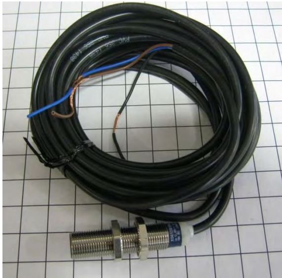
Image 5-14 – Meter roll proximity switch
