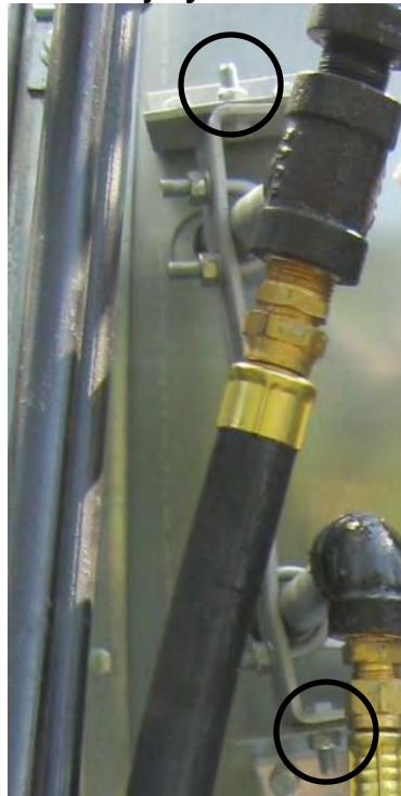
Image 3-1 – Vaporizer bracket on axial-fan dryer
