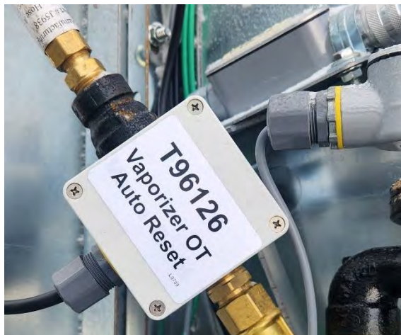
Image 4-11 – Vapor over-temp switch (shown on axial-fan dryer)
