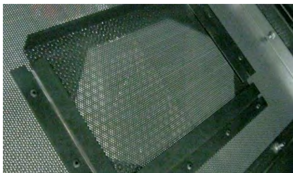
Image 4-44 – Inner grain column cleanout door
