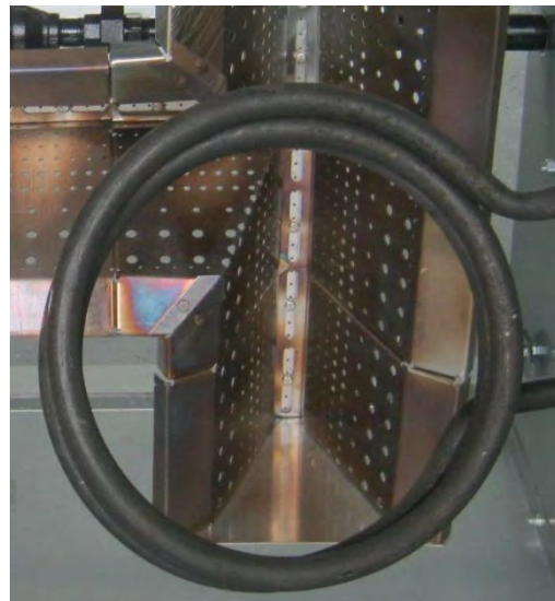
Images 4-32 & 4-33 – Vaporizer coil (shown on octagon burner, left, and on H burner, right)
