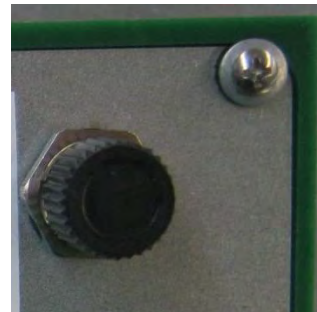
Image 4-49 – Cable connector capped
