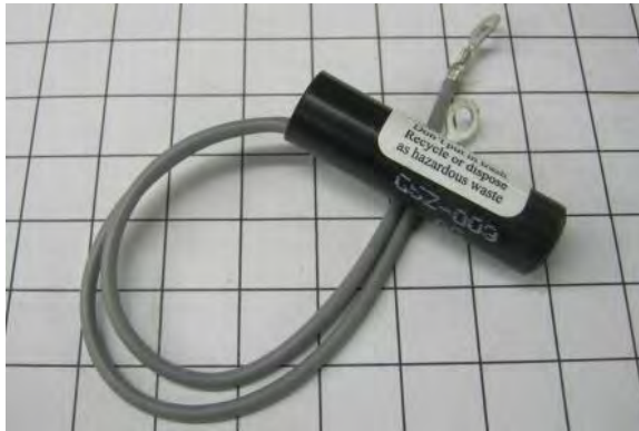
Image 5-1 – Grain discharge chute tilt switch
