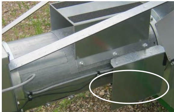
Image 4-1 – Discharge moisture sensor location
