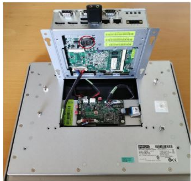
Image 2 – Battery location (circled)
