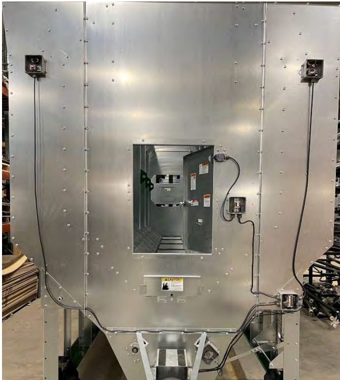
Image 5 - Back of mixed-flow dryer cooling section
