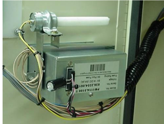
Figure 2.2b: Paper Roller Installed
