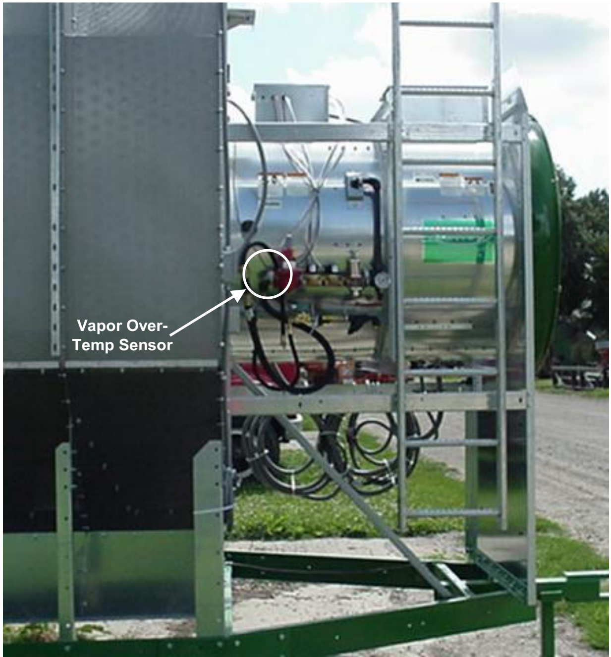
Figure 1.4c: Vapor Over-Temperature Sensor Installed on Dryer
