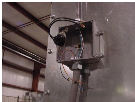
Photo 1.3: Removal of right front column high limit
