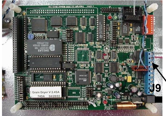
Photo 1.12: Processor board once the I/O board is removed. J9 is labeled and an arrow shows position 8.
