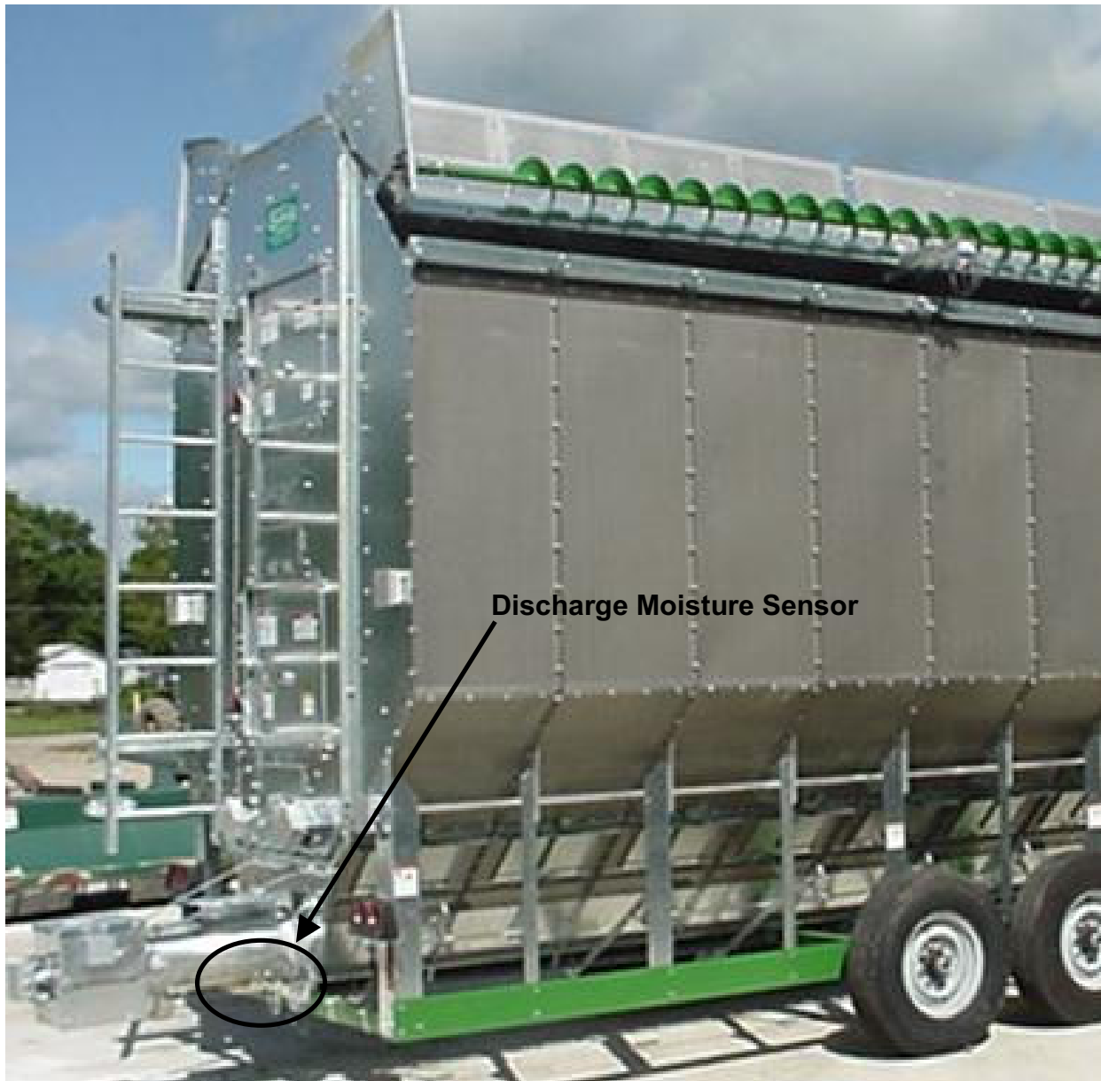
Figure 2.1c: Discharge Moisture Sensor Installed on Dryer
