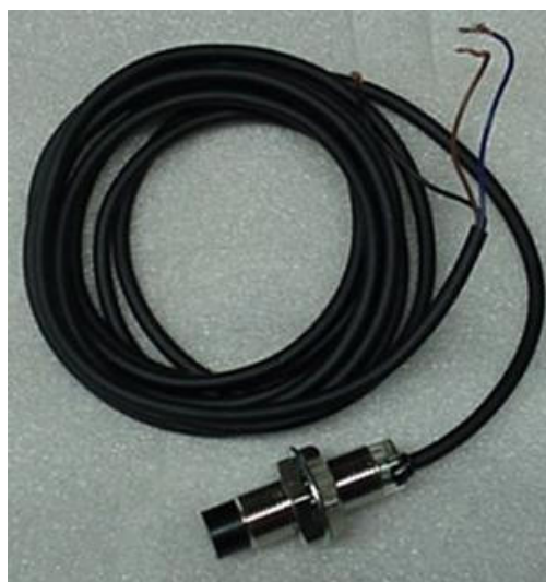
Figure 1.8b: Metering Roll Proximity Switch
