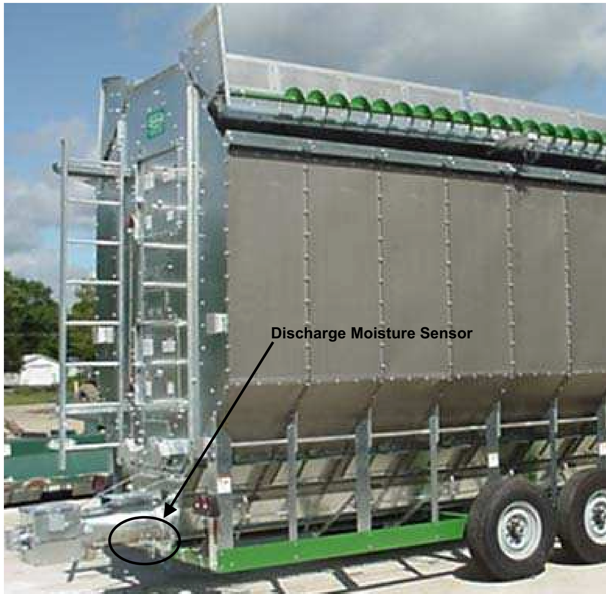
Figure 2.1c: Discharge Moisture Sensor Installed on Dryer
