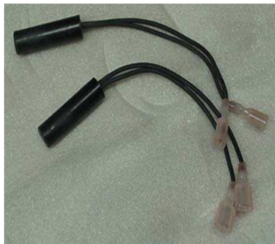
Figure 1.2b: Grain Level Sensor
