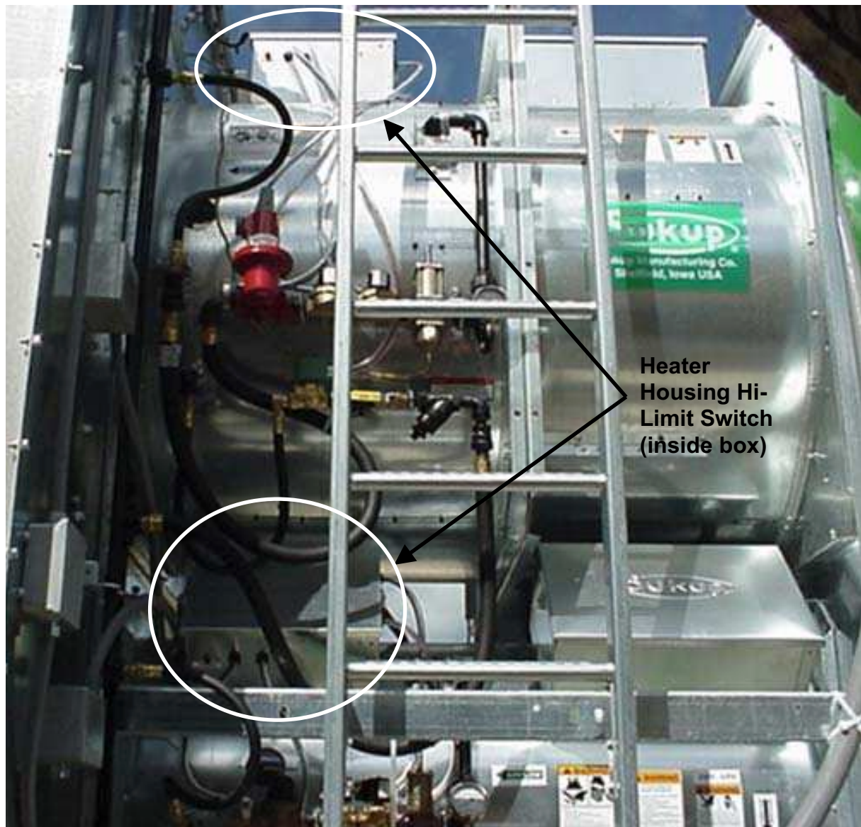
Figure 1.7c: Heater Housing Hi-Limit Switch Installed on Dryer
