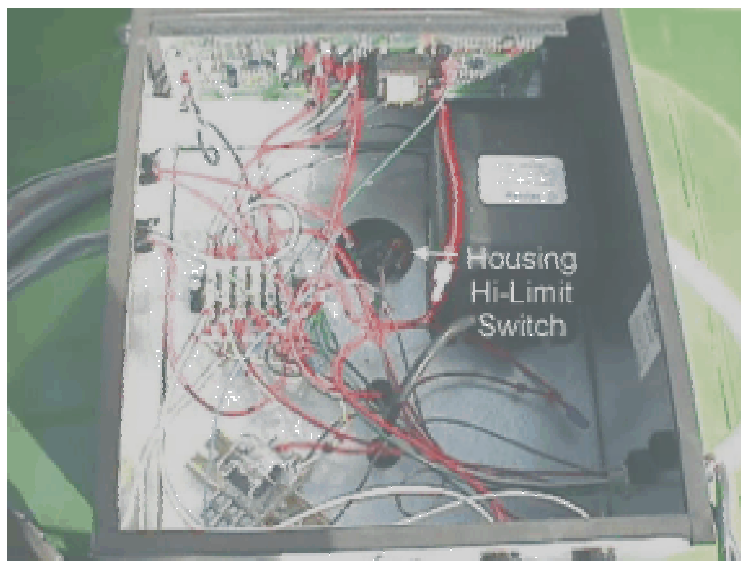
Figure 1.7c: Heater Housing Hi-Limit Switch Installed on Dryer
