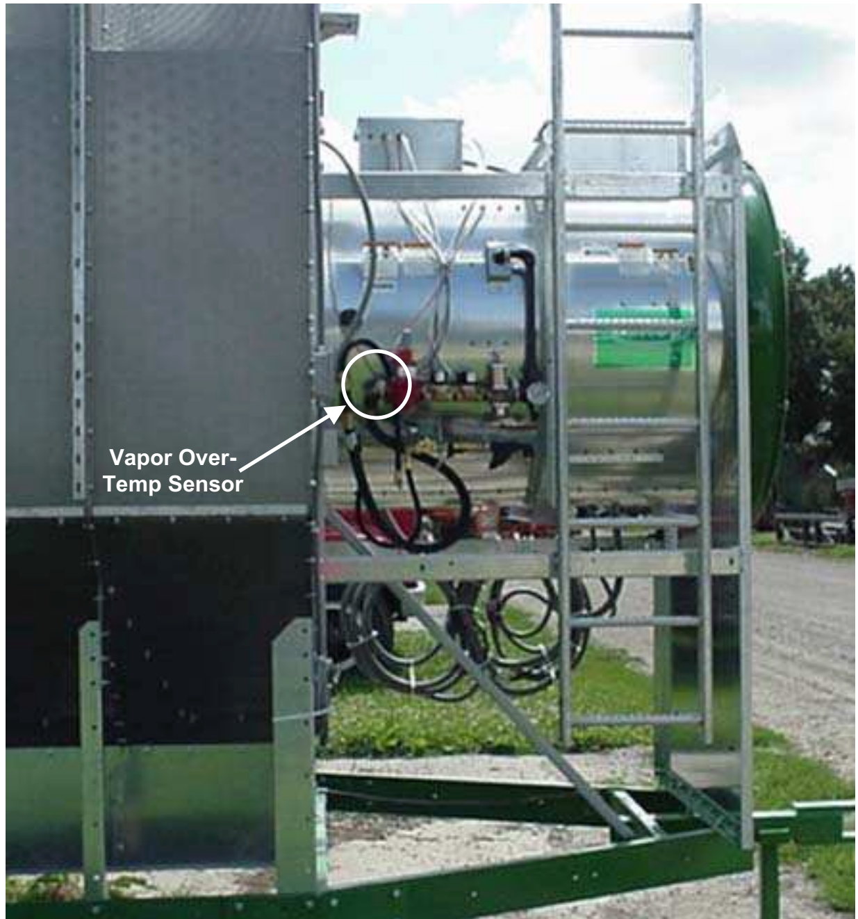
Figure 1.4c: Vapor Over-Temperature Sensor Installed on Dryer
