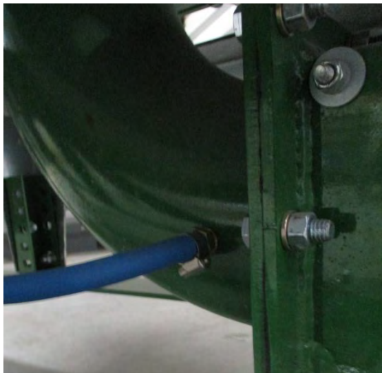
Image 3 – Air pressure sensor hose connected to blower outlet
