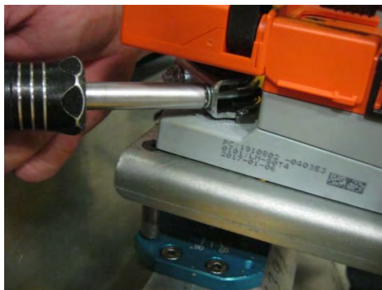
Image 6– Loosening butterfly valve collar
